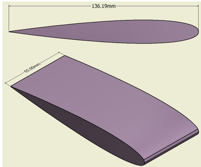
Figure 3: Hydroplane NACA0012 profile section and 3D model.
