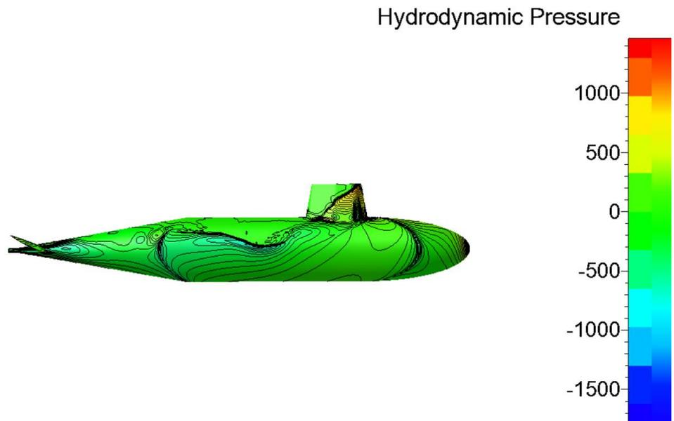
Figure 12: Hydrodynamic effect of submarine with hydroplanes (free motion and AoA 25 deg)
