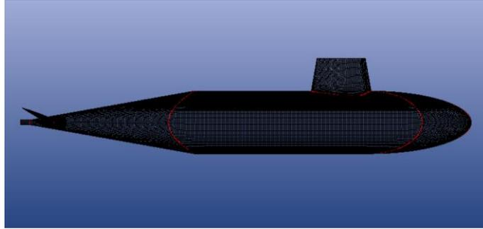
Figure 7: Generated mesh of the whole model.
