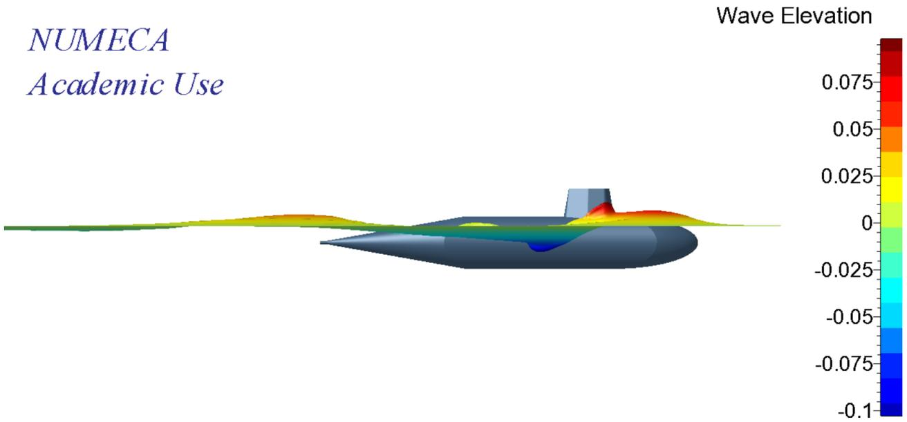
Figure 9: Wave elevation of submarine without hydroplanes (fixed trim)
