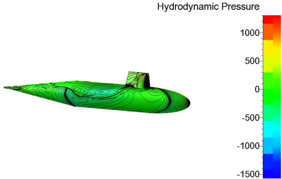
Figure 11: Hydrodynamic effect of submarine with hydroplanes (free motion and AoA 0 deg)
