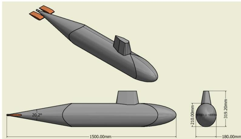
Figure 1: Model of submarine with hydroplanes.
