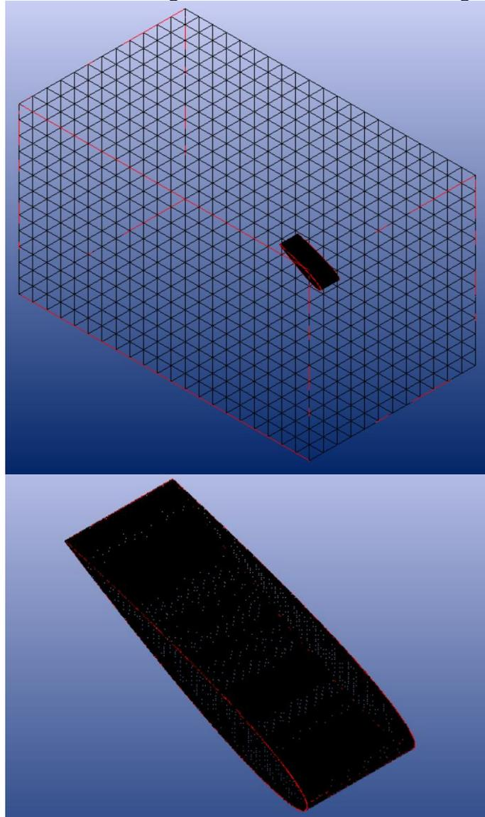
Figure 5: Generated mesh of the hydroplane(NACA0012).
