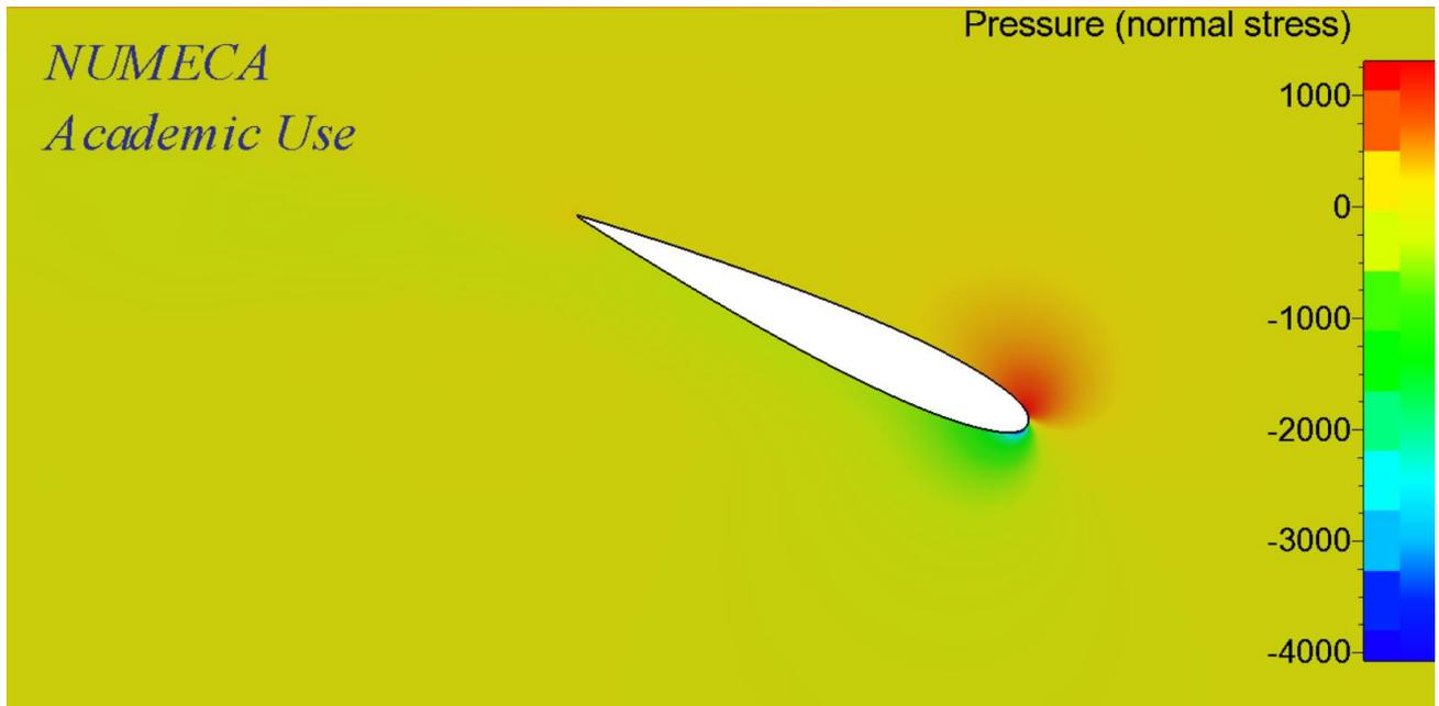
(a) Pressure distribution around the hydroplane.
