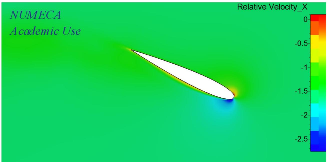
(b) Velocity distribution around the hydroplane.
