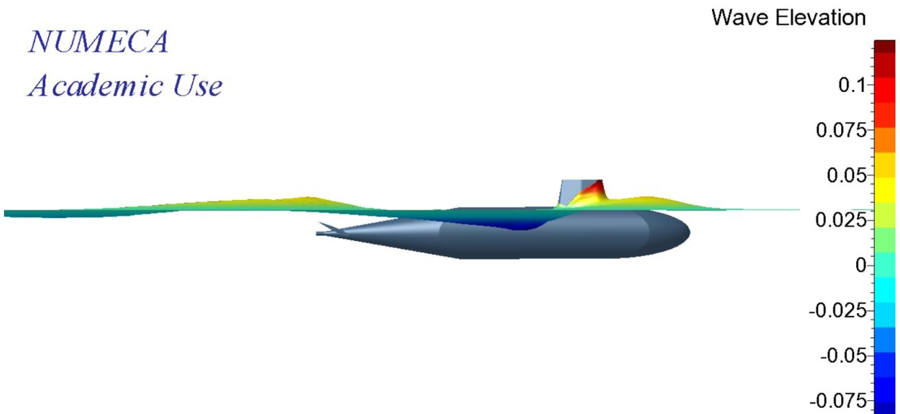
Figure 10: wave elevation of submarine with hydroplanes (free motion)
